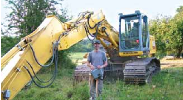
A 21-ton excavator used to create amphibian ponds in Schleswig-Holstein, Germany (David Orchard)
